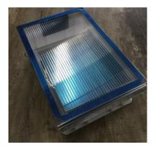
5. Place melter in a bright sunny level location on a warm day. Allow several hours for wax to start melting and check progress periodically. Change wax filled catch basins and clean metal pan of debris when needed. For large or heavy dirt batches, it may take more than one day to process the wax.
