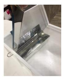
4. Rotate the screen/baffle so that it "points" up into the pan. The weight of the screen holds it against the pan's bottom. Add dirty wax, cappings, etc. to the pan and place the solar cover on top of the box.
